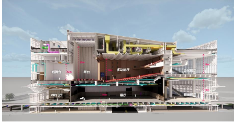
Fig.3 Net Spatial Clearances and Pipeline Layouts in Various Zones
